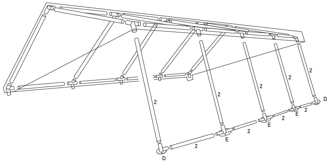
Attach the legs, feet and ground bars on the opposite side, then attach the ground bar on the two remaining sides. Once complete, peg down the structure.
