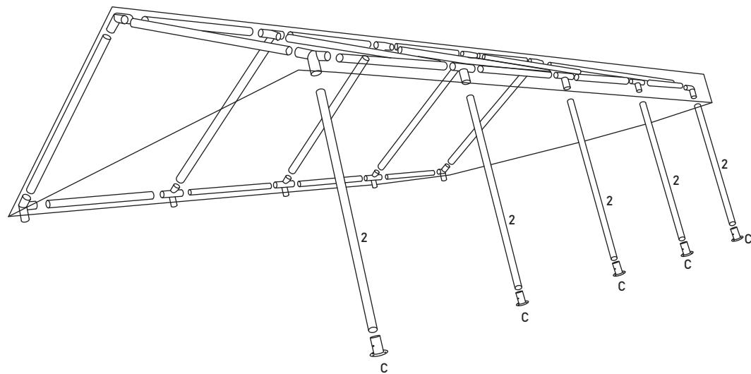
Attach the legs and feet on the other side then peg down the structure.
